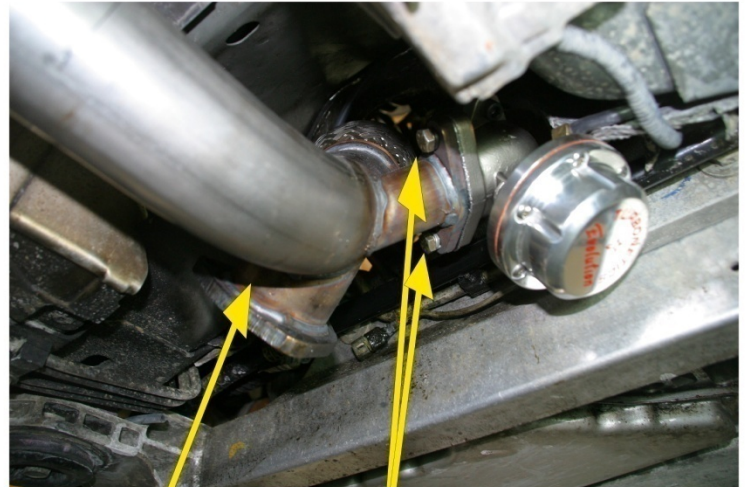
Tighten 13mm Bolts and Lockwashers
