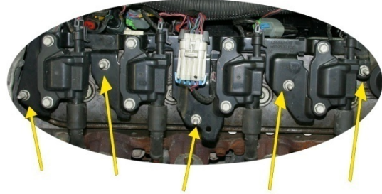
Remove these on rear valve cover for better spark plug access
