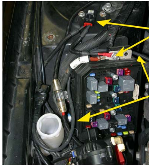
Vacuum Line To Vacuum Distribution Block
